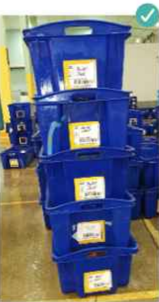
Maximum stack height: 5 x Large crates without pallet
