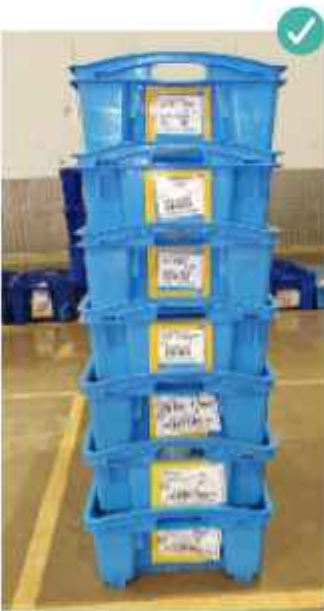
Maximum stack height: 7 x Small crates without pallet
