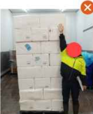
Pallet height more than 1.2m. Pallet should be double stacked.
